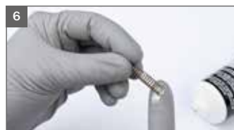
6 Grease and insert paint needle spring
