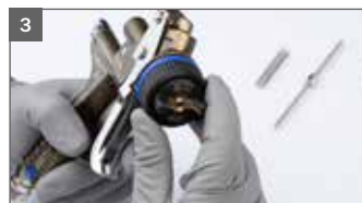
3 Assembly of the air cap
