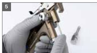
5 Insert paint needle
