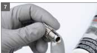
7 Grease thread of material flow control screw
