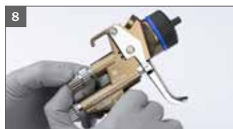
8 Install material flow control screw
