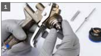
1 Assembly of the fluid tip
