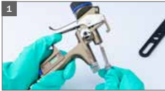
1 First remove paint needle.
